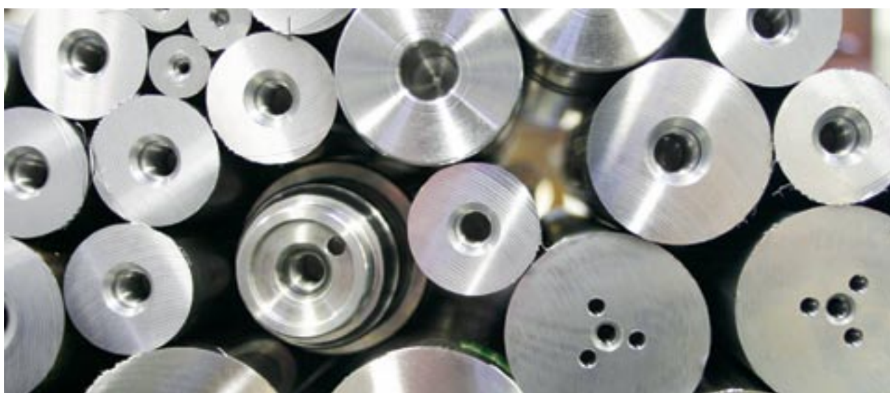
Photo below: Machined rotor shafts with a variety of centre bores and drill hole patterns
