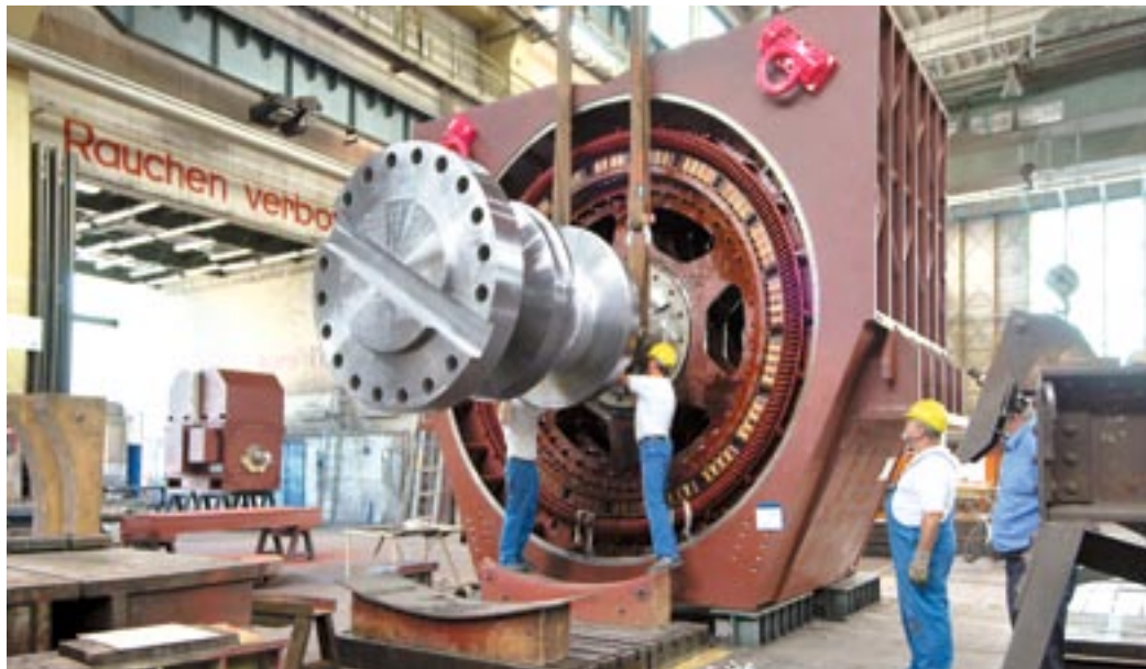
Photo: Karin Wagner Millimetre clearances: Insertion of the giant rotor into the stator calls for ultimate precision.
