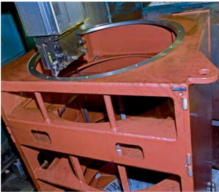
Machining of a generator housing on the CNC carousel
