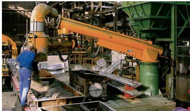
Mixer line with continuous mixer (30 t/h) in the hand moulding shop
