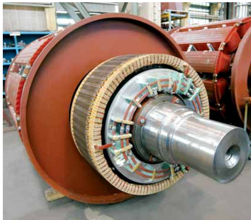
This rotor with exciter for a synchronous generator is destined for a ro-ro ferry in Canada.
