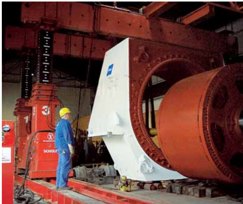
A 6 MW synchronous motor for a blooming stand drive: one of the top-quality products from VEM Sachsenwerk.
