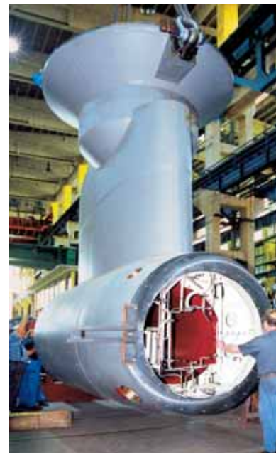
A Sachsenwerk machine for the shipbuilding industry: a unit known as a POD drive enables cruise ships to manoeuvre in the restricted space of harbour basins.
