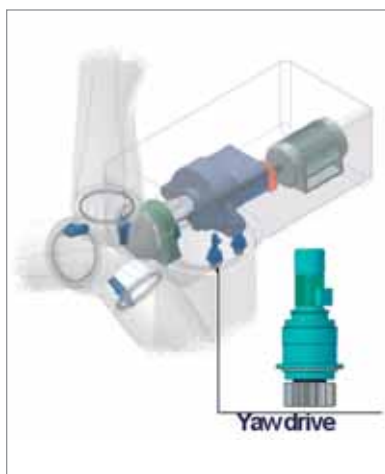
Above: The nacelle is turned with four drives. Right: B21R 112 MX 6 with cycloidal precision gearing.
