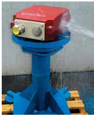
Fig. 1: Test setup for the jet water test for protection type IP X5
