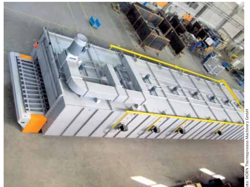
A pattern burning machine in which patterns are attached to bottles and other types of glass
