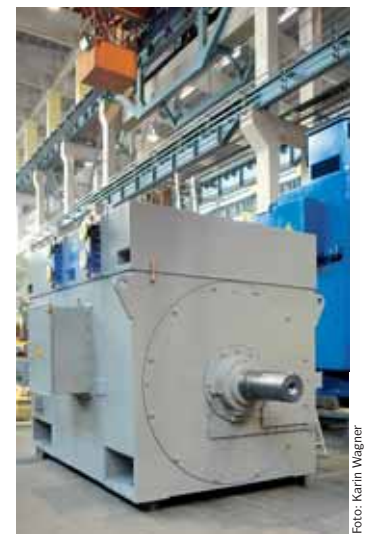
Slip ring rotor motor with KBAV, 45 MW; 6kV
