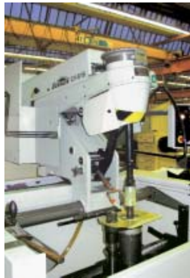
Cross-grinding of the bores
