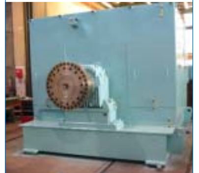
Synchronous generator for the cruise liner "Pride of America"
