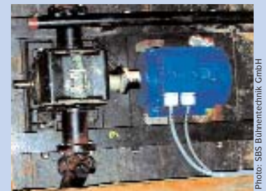
Under the boards: Wagon stage drive at the Semper Opera House
