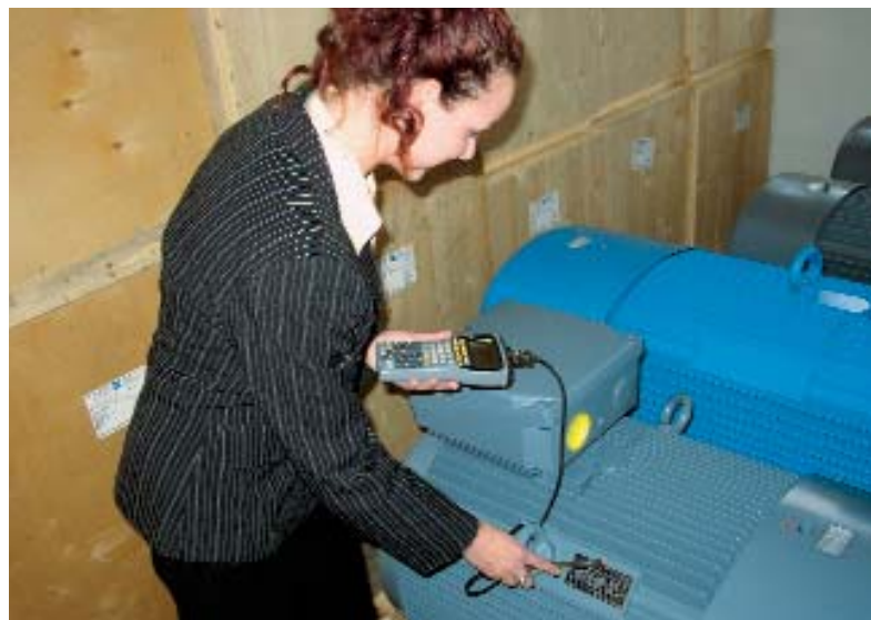
Michaela Möser of the overseas export department demonstrates the electronic label of a memory motor
