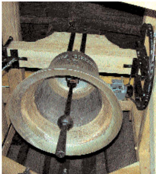
The four-bell peal in Dohna was equipped with motors with shaft heights between 71 and 90 mm.
