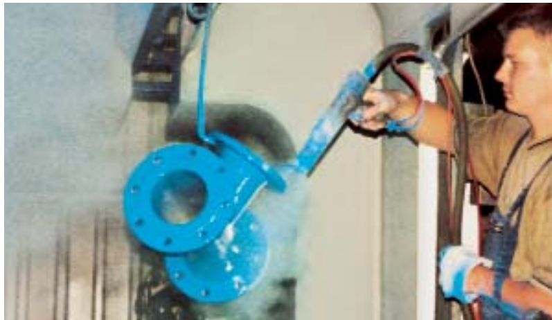
High-quality, environment-friendly surface treatment for castings
