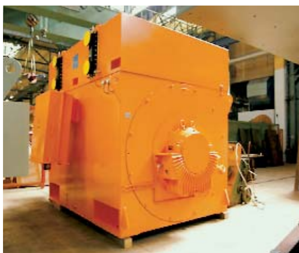
Induced draught fan drive with 8 MW, 11 kV asynchronous motor for Cottam Power Station (UK)
