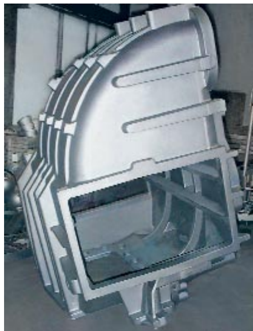
Charger-air cooling for M 43C marine diesel engines
