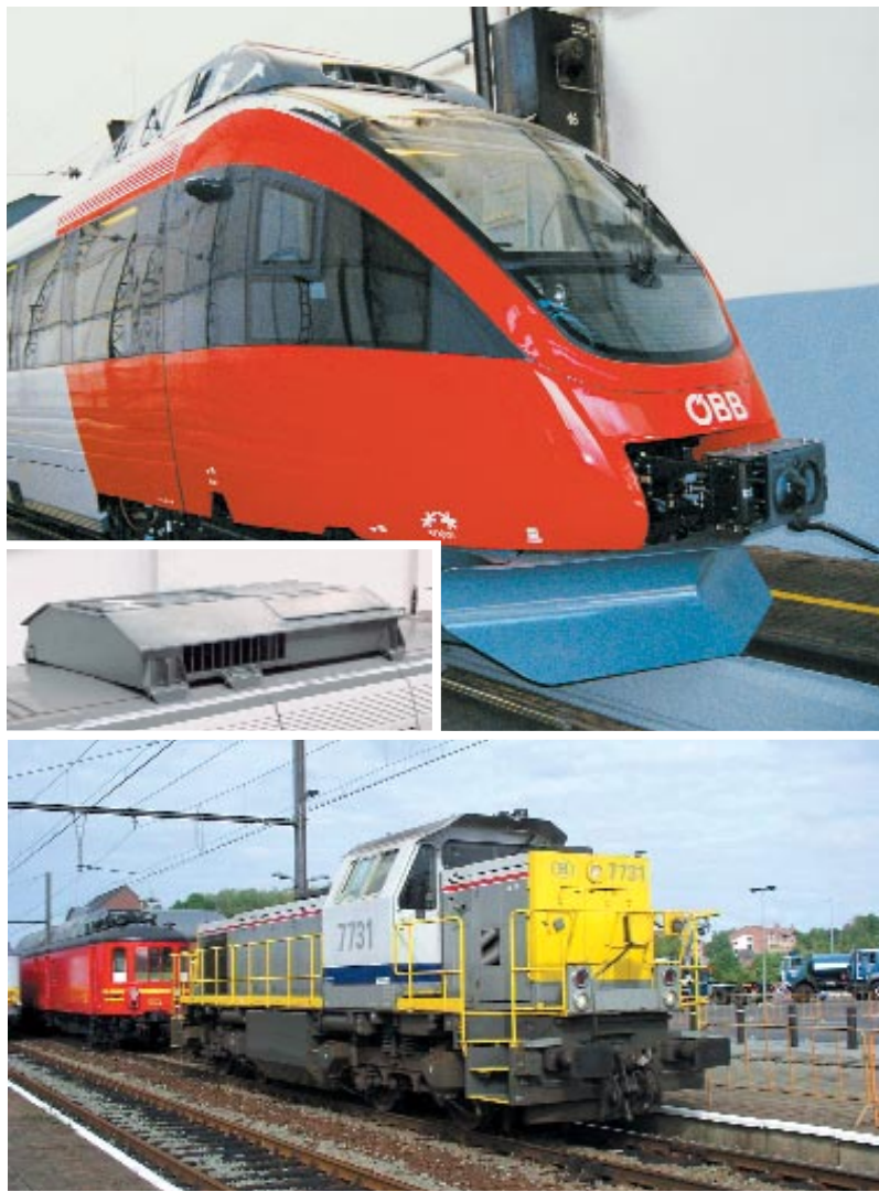
A high-speed train of the Austrian Federal Railways (above). The roof section houses the VEM auxiliary drives (centre). The new diesel-hydraulic locomotive HLD 77C (below).
