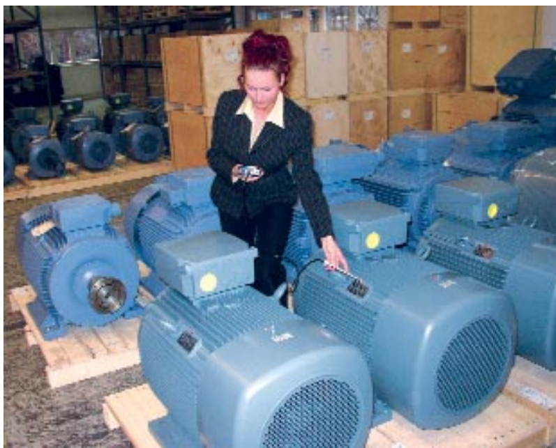
RFID technology makes it possible: Important data can be stored and retrieved at the motor itself.
