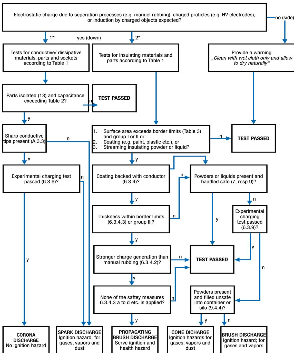
Bild 1.6: IEC/TS 60079-32-1, Figure F.1 – Flowchart for a systematic electrostatic evaluation with reference to the respective chapters
