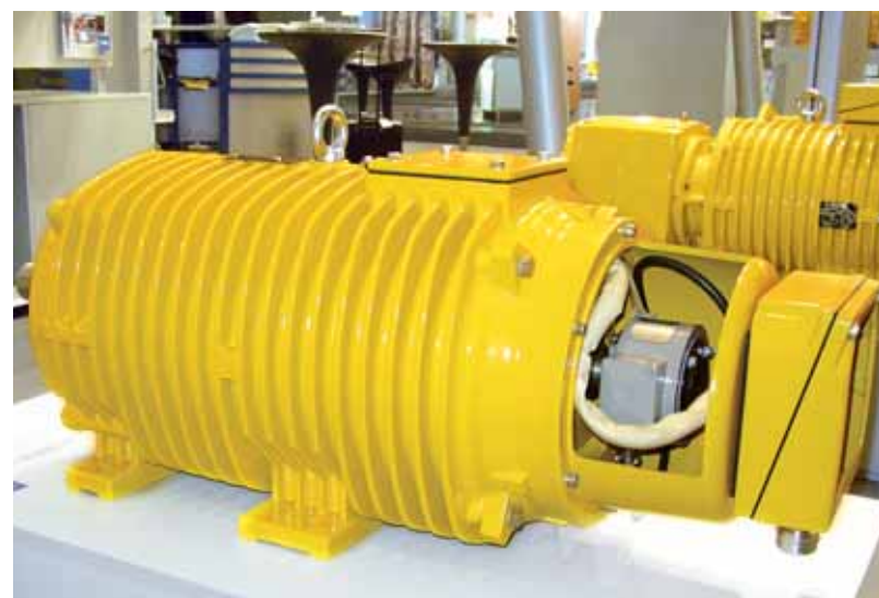
Fig. 3: 5.80 kW roller table motor with hooded encoder and terminal box mounted at the N end
