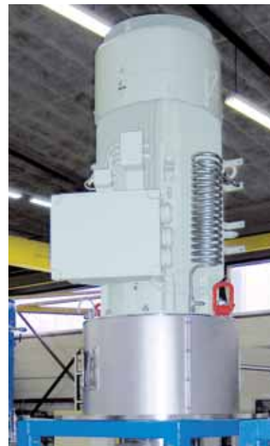
Fig. 2: Special motor for liquid-gas pumps, frame size 355
