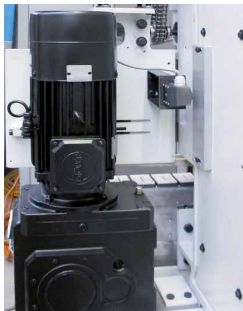
A VEM motor with mounted gearbox for a wood-processing machine.
