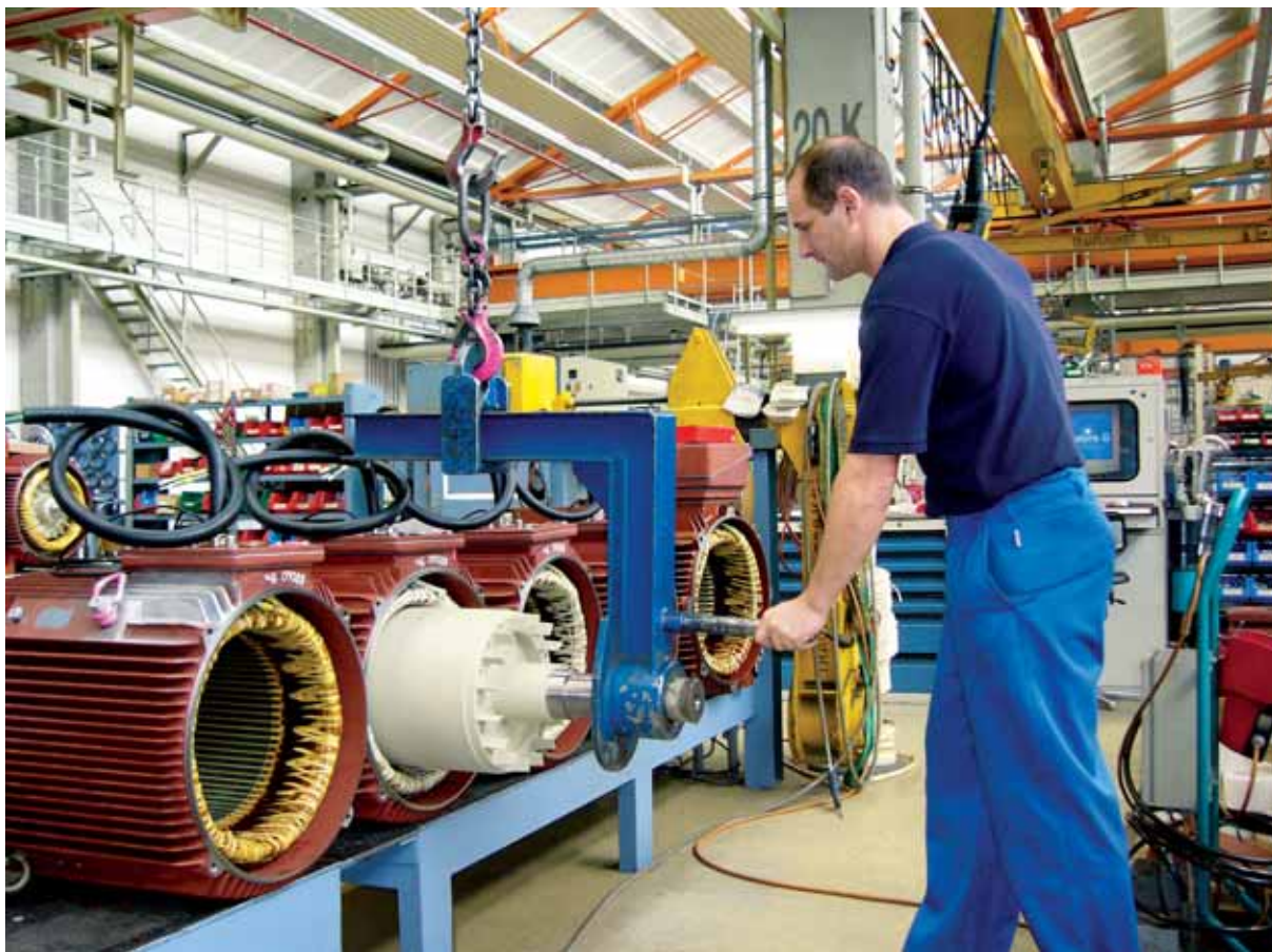
continued on page 2 Engineer Olaf Giese inserts a rotor into its stator. The motor belongs to the fans for a tunnel ventilation system.
