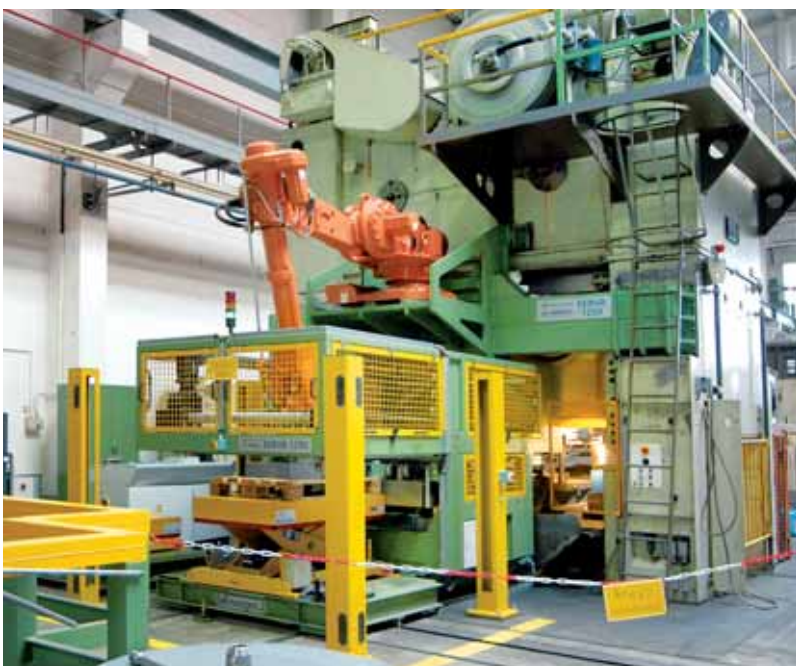
The strip processing plant in the press room has been upgraded with an industrial robot.
