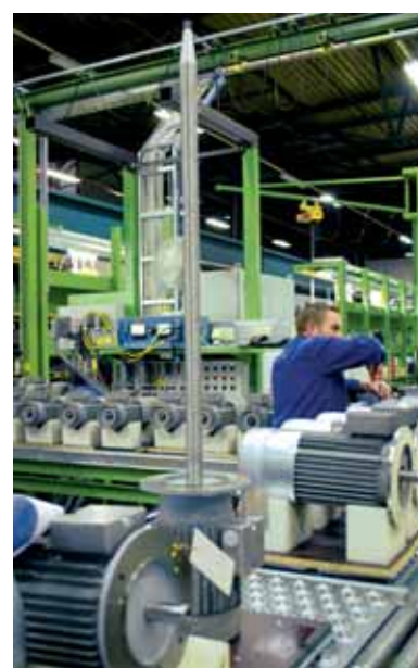
Fig. 4: Thomas Gottschlich testing special motors for use in agitators, as brake motors in wind turbines or for installation onto gearboxes
